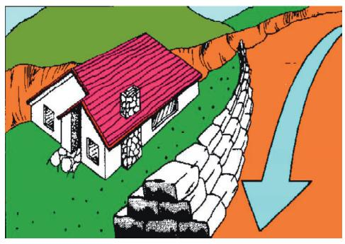
MUD AND DEBRISFLOW DIVERTED BY SANDBAGS
